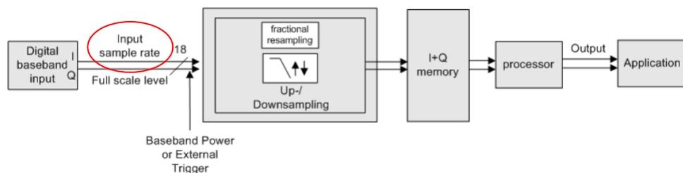
**Figure 39: Digital baseband acquisition hardware of the R&S FSV**
