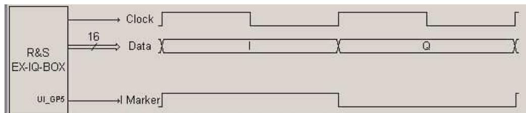
**Figure 21: Marker timing for interleaved parallel data**
