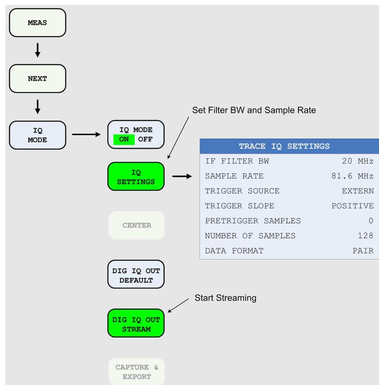
Figure 31: Analyzer configuration for IQ streaming
