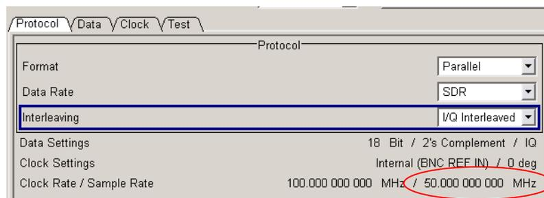
**Figure 16: Indication of calculated Sample Rate**
