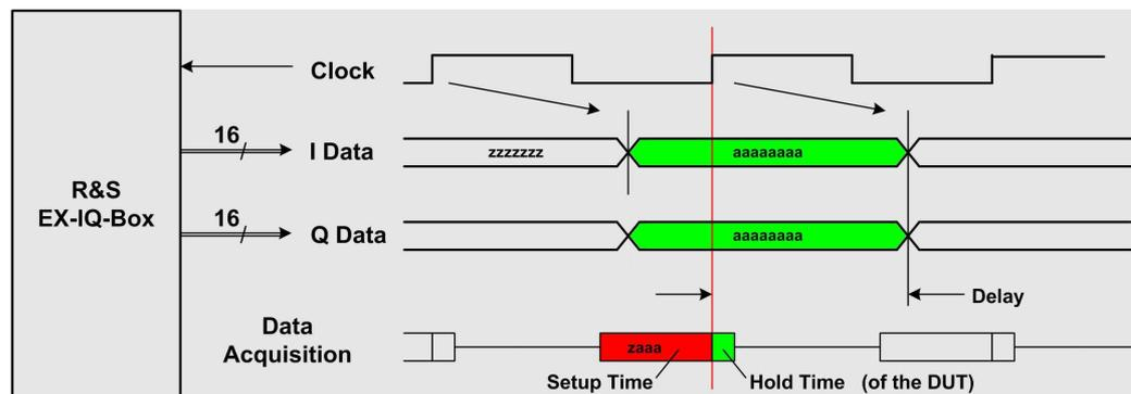
Figure 63: Delay + setup time reaches clock period
