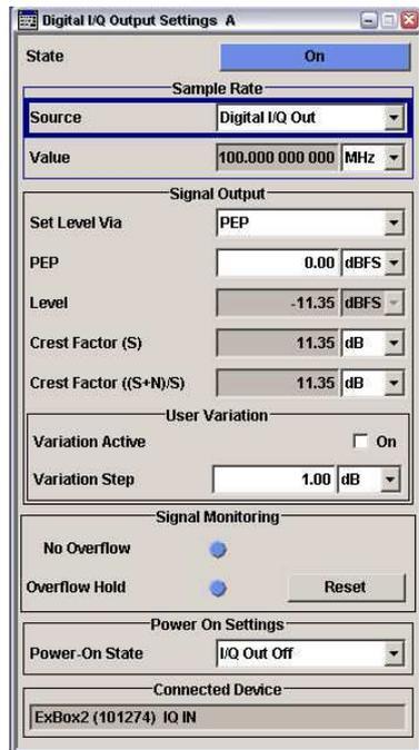
Figure 25: Configuration of the digital I/Q output
