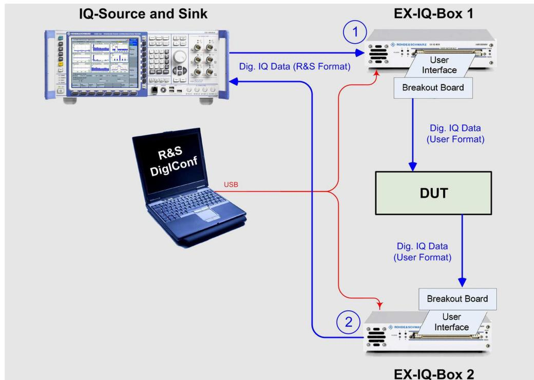
**Figure 5: DUT between the R&S CMW's IQ input and output**
