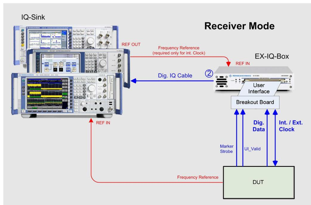
Figure 38: Instruments and signals in receiver mode
