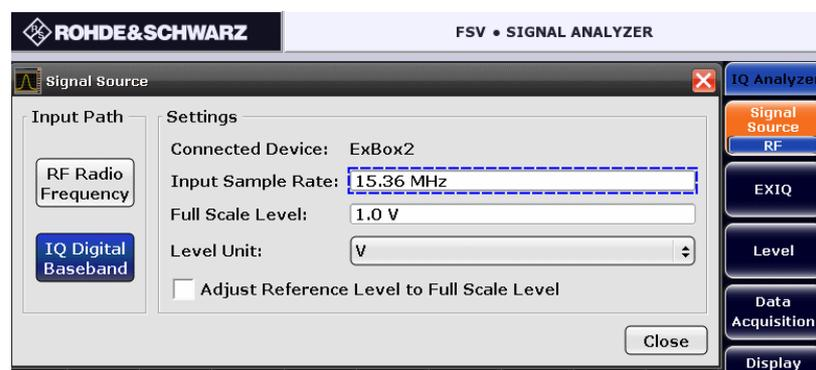
Figure 40: Select the signal input for the R&S FSV
