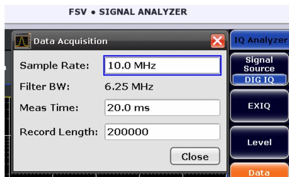
Figure 42: Setting of the fractional resampler
