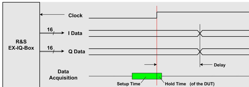
Figure 62: Case 3 - TX, external clock
