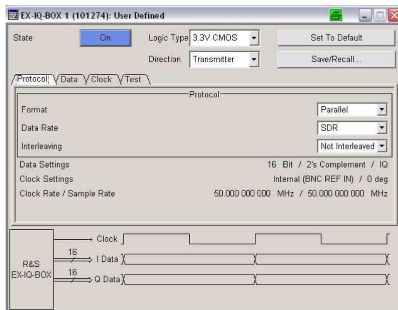
**Figure 12: Setting parameters for the Protocol tab**
