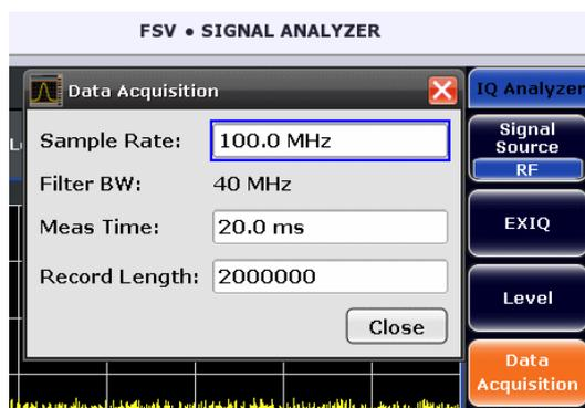
Figure 28: Output Sample Rate for streaming
