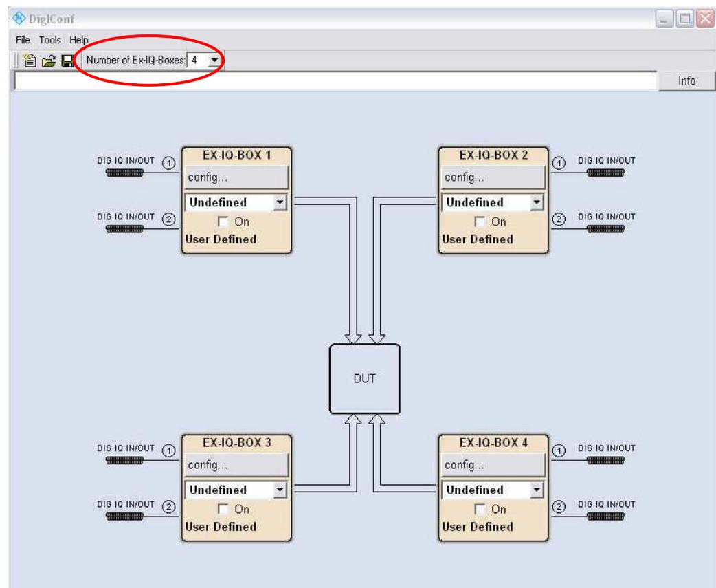
Figure 6: Top level of the *DigiConf* GUI, controlling up to four R&S EX-IQ-Boxes
