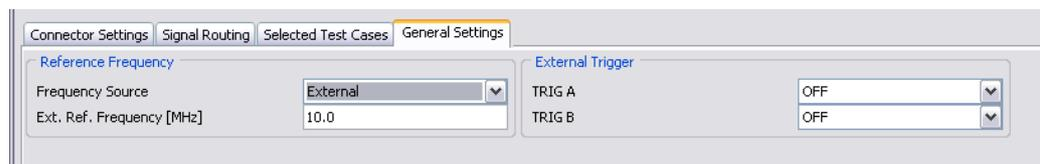
**Figure 36: Synchronization of the R&S CMW and DUT**
