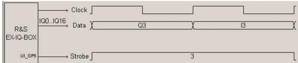
**Figure 22: Marker timing for Q/I interleaved serial data, bit position = 3**
