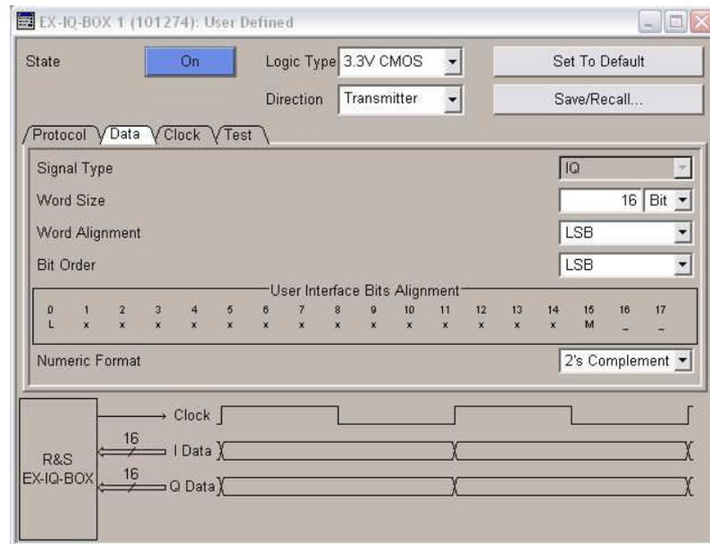
Figure 13: Setting parameters for the Data tab
