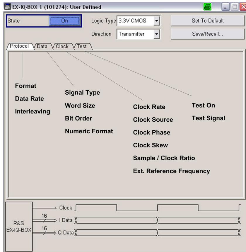
Figure 11: Setting the parameters of the main User Defined panel
