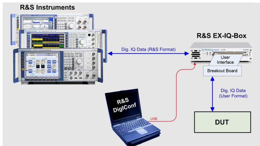
Figure 3: Basic operation of the R&S EX-IQ-Box
