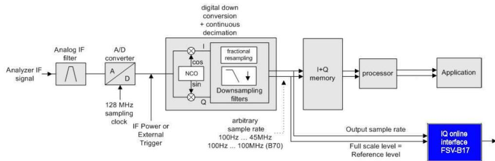
**Figure 26: Data acquisition hardware in the R&S FSV**
