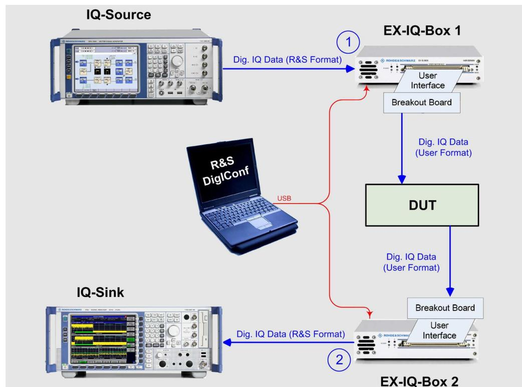
**Figure 4: DUT between an IQ transmitter and IQ receiver**
