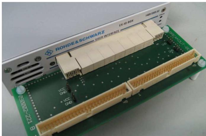
**Figure 69: Single-ended breakout board**
