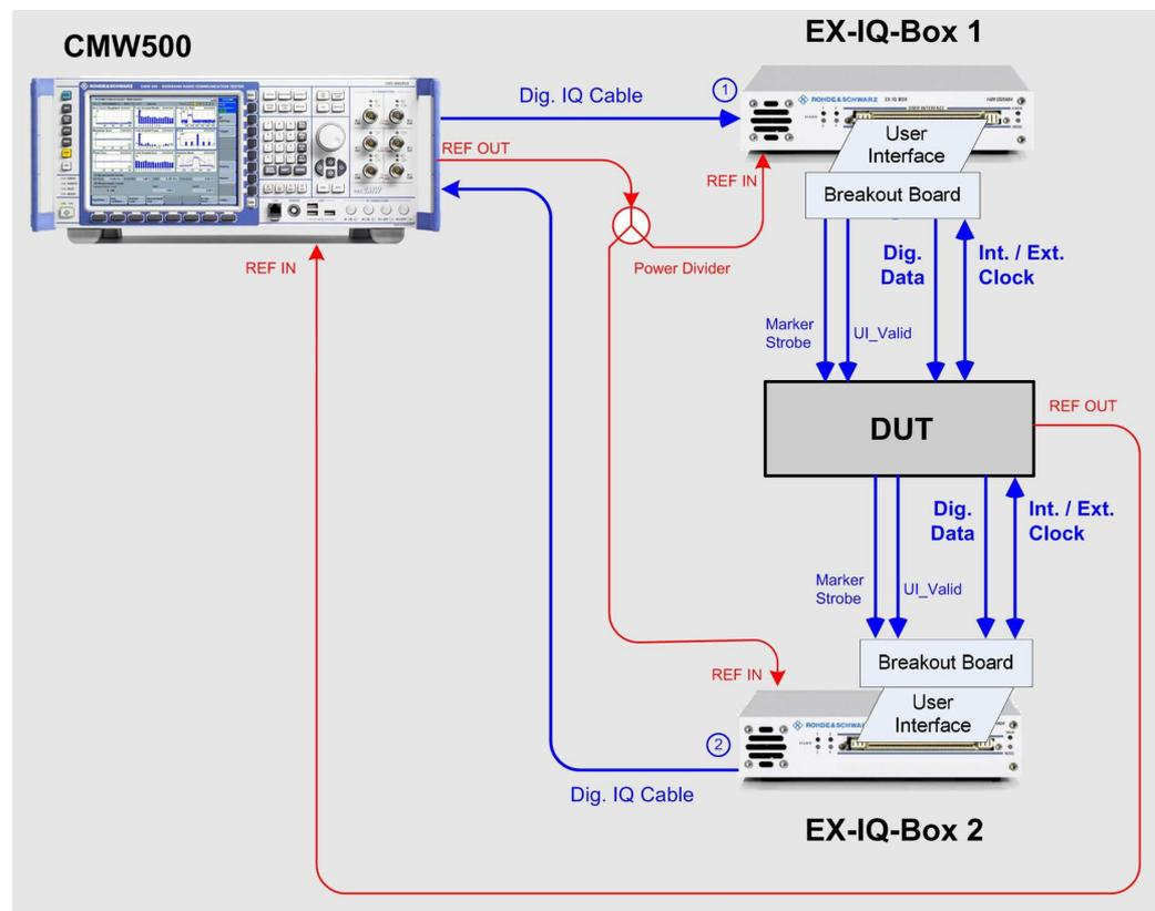
Figure 54: DUT between the R&S CMW's IQ input and output
