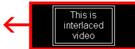
During the first 175 fields, the element scrolling to the left at four pixels per field using real interlacing (video) is inserted in the free tenth line of the film area (5.1.1).
