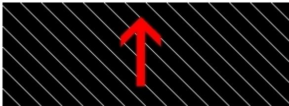
On an area of 420x105 pixels, white, one-pixel-wide 45° diagonals scroll upwards at a spacing of 20 pixels and a speed of one pixel per field. Pixels that leave the area are reinserted at the bottom. After 420 fields, the start position is reached for the fourth time, and this position is maintained for the final 100 fields.
