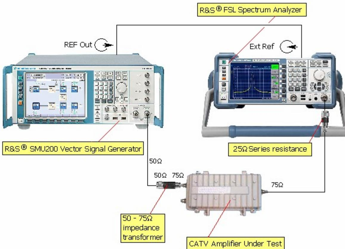
Figure 13 Test set-up for IMD test
