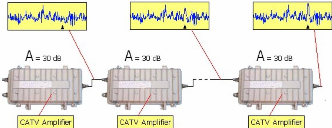
*Figure 10 Cascading effect of amplifiers*
