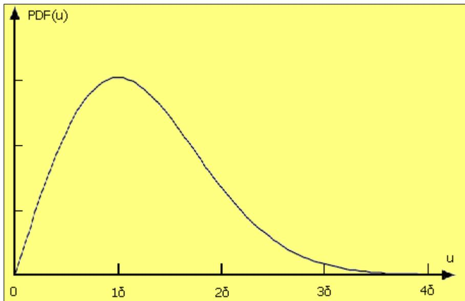
*Figure 11 Amplitude distribution of Gaussian noise*
