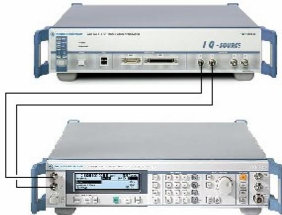
*Figure 20 AFQ100A/SMV03 combination as an alternative to SMU200A*
