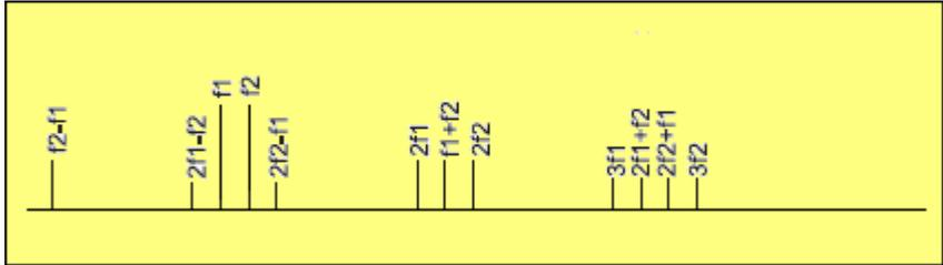
*Figure 3 “Two-tone” 2<sup>nd</sup> & 3<sup>rd</sup> order intermodulation products for device with 1<sup>st</sup>, 2<sup>nd</sup> & 3<sup>rd</sup> order terms in its transfer function*
