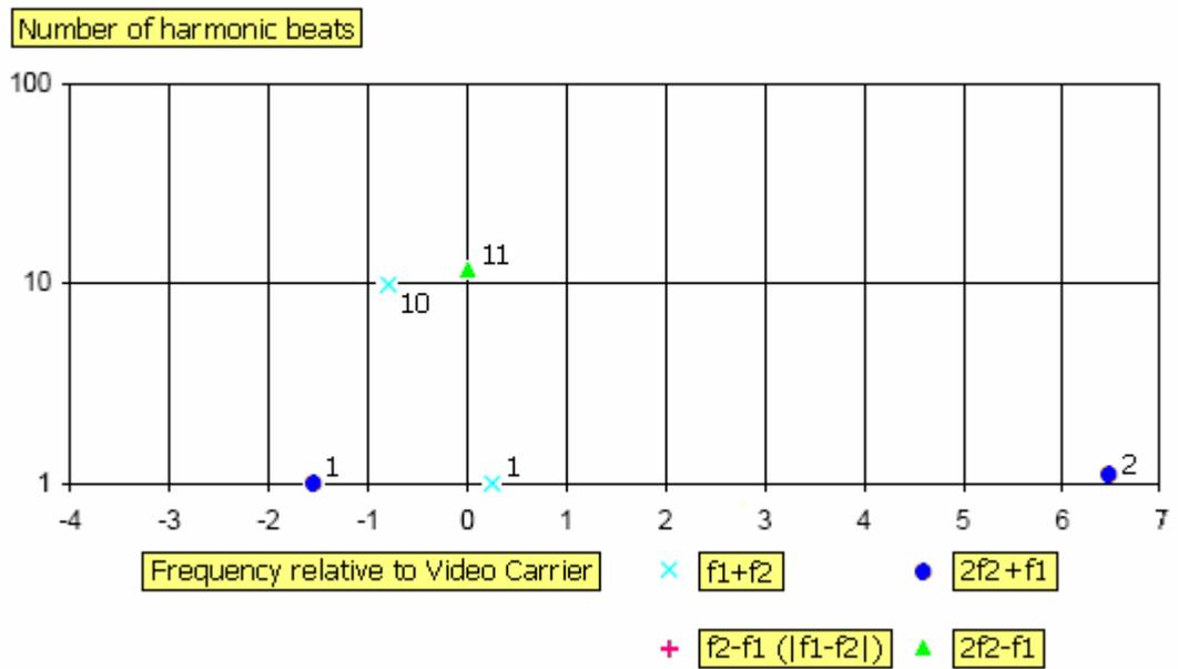
*Figure 5 Some important 2<sup>nd</sup> & 3<sup>rd</sup> order harmonics of EN50083-3 test carriers @ upper band edge UHF channel 69 or 855.25 MHz*
