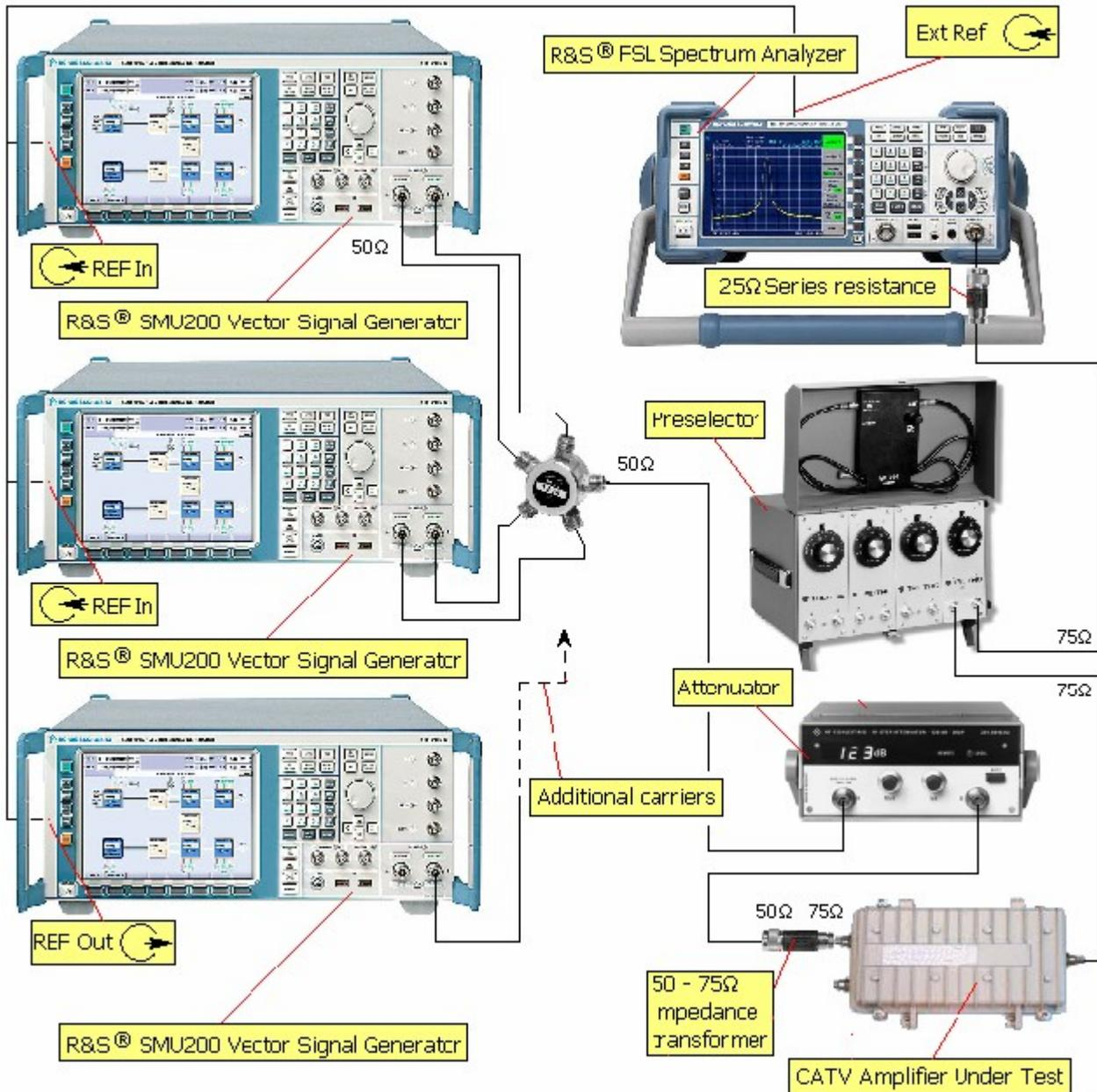
Figure 26 Test set-up for XMOD test
