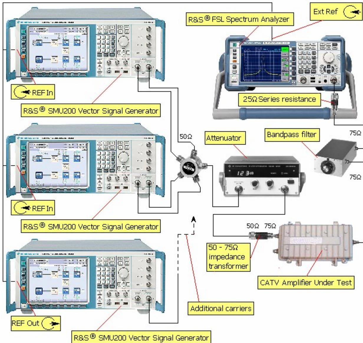
Figure 25 Test set-up for CBT measurement
