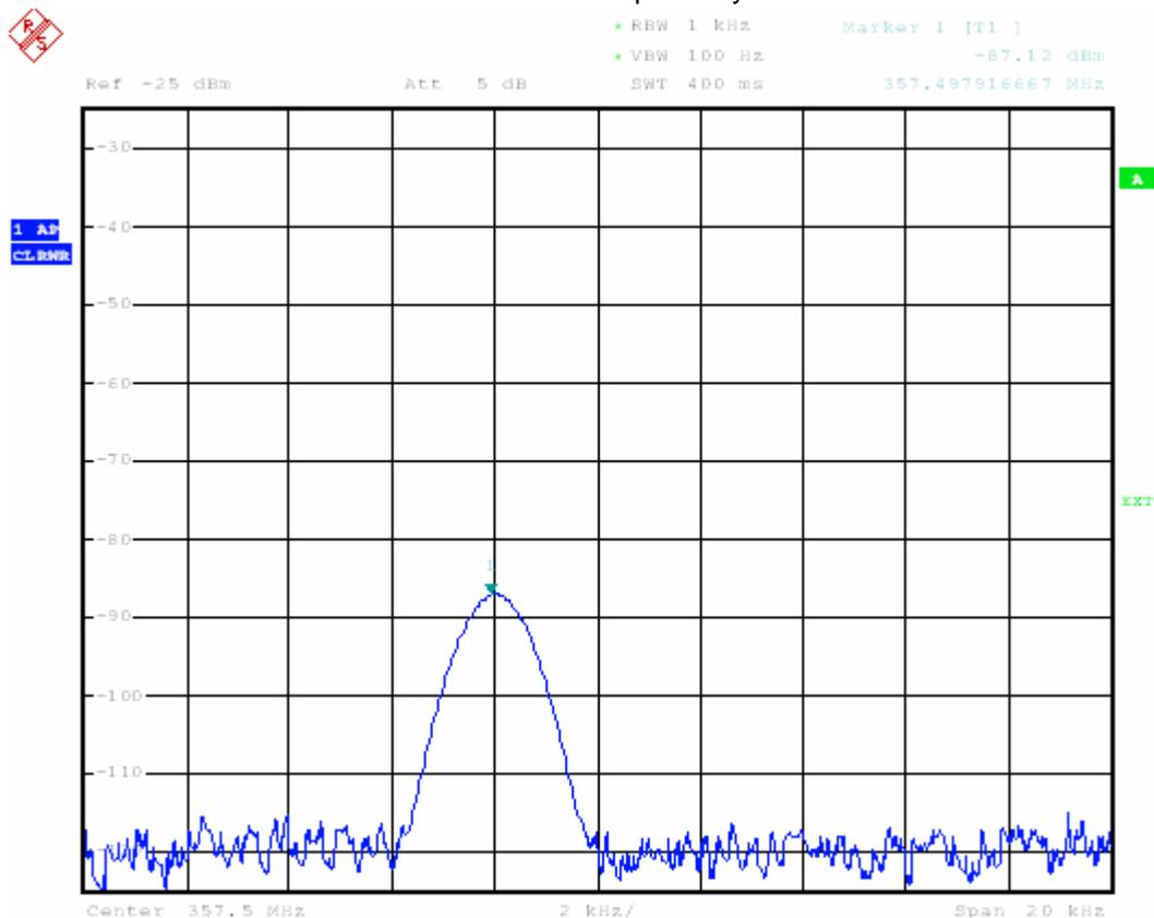
Figure 18 Intermodulation component
